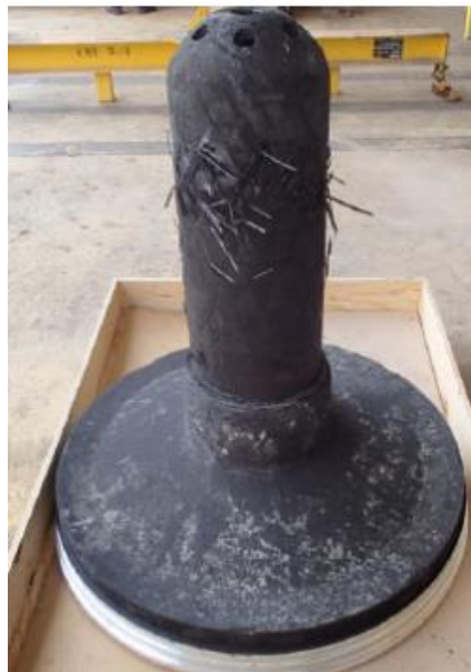
The Igniter after a static motor firing test
