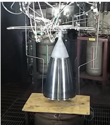
LEROS 2c engine in test
