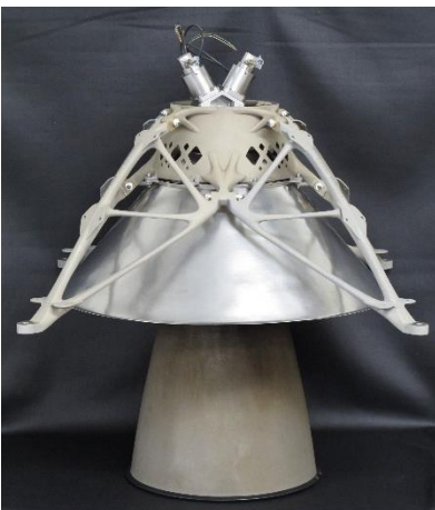
LEROS 2b with heatshield and Additive Manufactured support structure.
