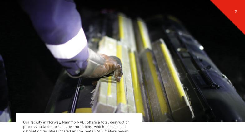
Our facility in Norway, Nammo NAD, offers a total destruction process suitable for sensitive munitions, which uses closed detonation facilities located approximately 900 meters below the surface in a disused copper mine. Typically, Nammo NAD can process up to 2.5 tons Net Explosive Quantity (NEQ) per day, making this a unique and extremely fast process.
