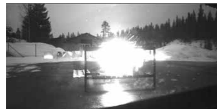
High speed camera photo of a detonating APEX round in a light-skinned - i.e. 2mm DurAl plate multi-array target. Photo: Alexander Kralic
